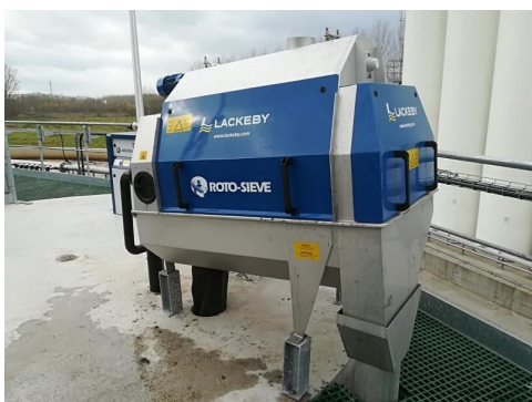
Roto-Sieve rotating drum screens
